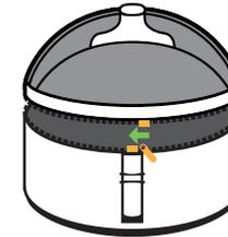
Insert zipper pin on the carrier lid into the zipper box on the base. Make sure pin is fully inserted.
