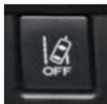
Press and hold this switch for two seconds to turn off the Lane Departure Warning and the Lane Sway Warning functions.
