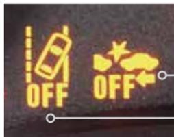
When these functions are off, the indicator light on the instrument panel illuminates.
