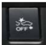
Press and hold this switch for two seconds to turn off the Pre-Collision Braking System and Pre-Collision Throttle Management.
